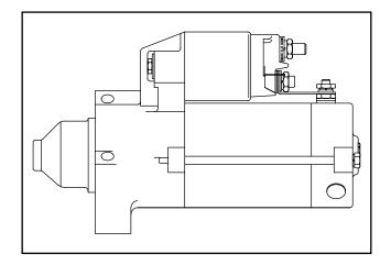
Figure 10. Starter Motor (V-Twin Engines)
